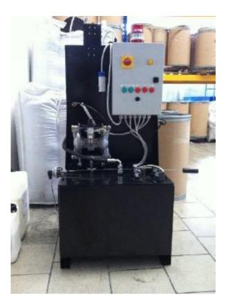
**LUBRO MIX** is a dosing unit for water-soluble release agents in aluminum die casting.
