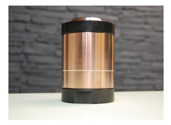
HGS TOP is a three part system made of high quality material. The treated steel on this plug insures a long life while the Beryllium copper piston prevents friction and adds to injection speed and heat exchange.
